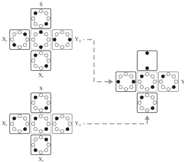
Fig. 8. The schematics of the structure proposed by Lebar Bajec *et al.* that implements the ternary AND and OR logic functions based on the principle of abrupt switching.
