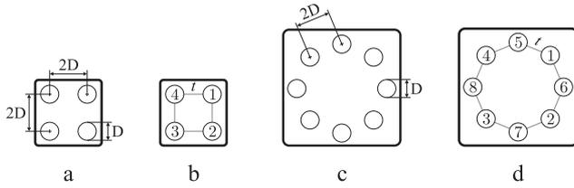
Fig. 1. The geometry of the binary quantum-dot cell presented by Lent *et al.* (a) and the denotation of the quantum dots and the tunnelling paths (b). The geometry of the ternary quantum-dot cell presented by Lebar Bajec *et al.* that was constructed by adding four additional quantum dots to the binary cell (b). The denotation of the quantum dots and the tunnelling paths in the ternary quantum-dot cell (c).
