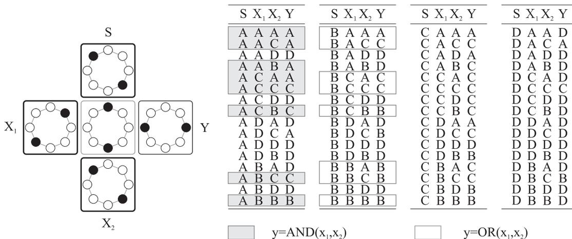
Fig. 7. The QCA based structure that was obtained by substituting the bQCA cells in the binary majority gate structure with tQCA cells (left). There are three input cells named S,  $X_1$  in  $X_2$ , and one output cell named Y. The structure's truth table for all possible combinations of input cells' states (right).
