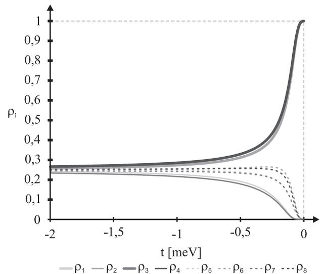
Fig. 5. The dependency of the single-electron density at individual sites,  $\rho_i$ , with respect to the tunnelling energy, for the case of a ternary quantum-dot cell transiting from neutral state to the state marked as A.
