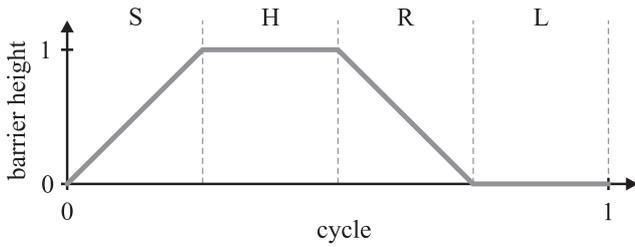
Fig. 3. The cyclic signal that controls the adiabatic switch is composed of four phases, namely: switch (S), hold (H), release (R), and relax (L). In the graph the barrier height is normalized to the interval [0, 1], where value 0 denotes lowered barriers (high probability of the electrons tunnelling between adjacent quantum dots) and value 1 denotes raised barriers (no tunnelling of electrons possible). The four phases are of equal length, thus each lasts 1/4 of the complete cycle.
