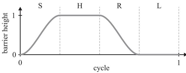
Fig. 6. The cyclic signal that controls the adiabatic switch in a ternary quantum-dot cellular automaton.
