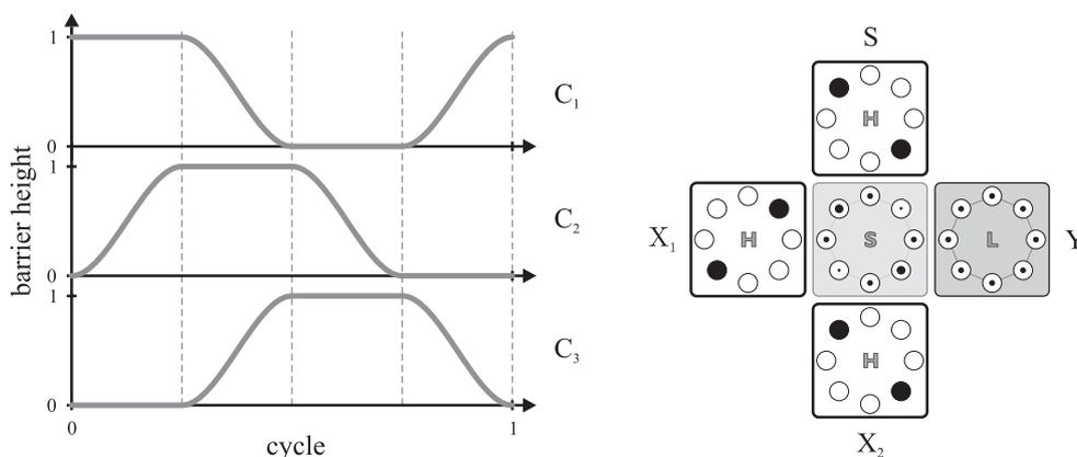
Fig. 9. The schematics of the structure that implements ternary AND and OR logic functions based on the principle of adiabatic switching. Cells marked with H (hold phase) are controlled by the cyclic signal  $C_1$ , those marked with S (switch phase) by  $C_2$  and those marked L (relax phase) by  $C_3$ . A close inspection reveals that the size of the structure corresponds to the size of the structure, which implements the binary AND and OR logic functions.
