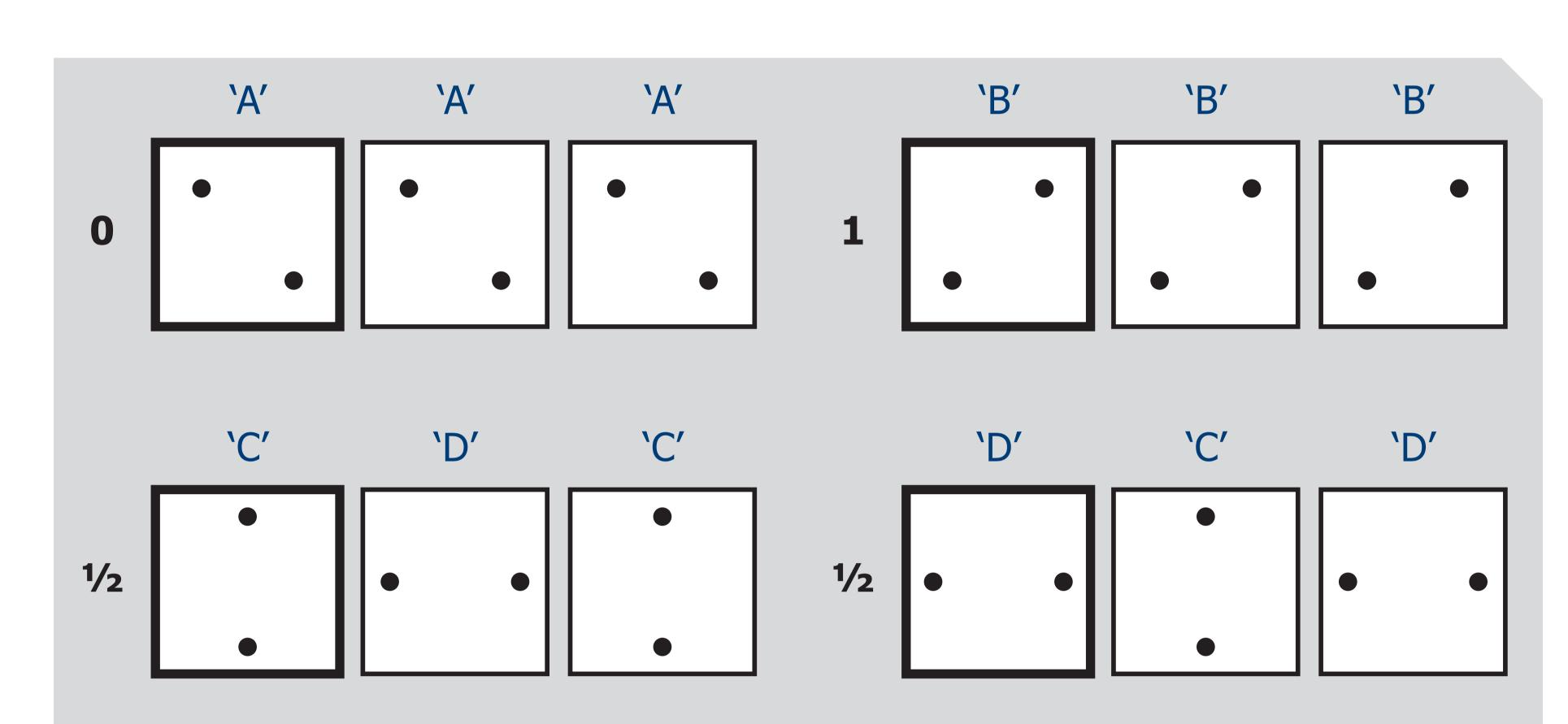
The three-state wire. Propagation of logic values 0,  $\frac{1}{2}$  and 1 over a line of extended quantum-dot cells.
