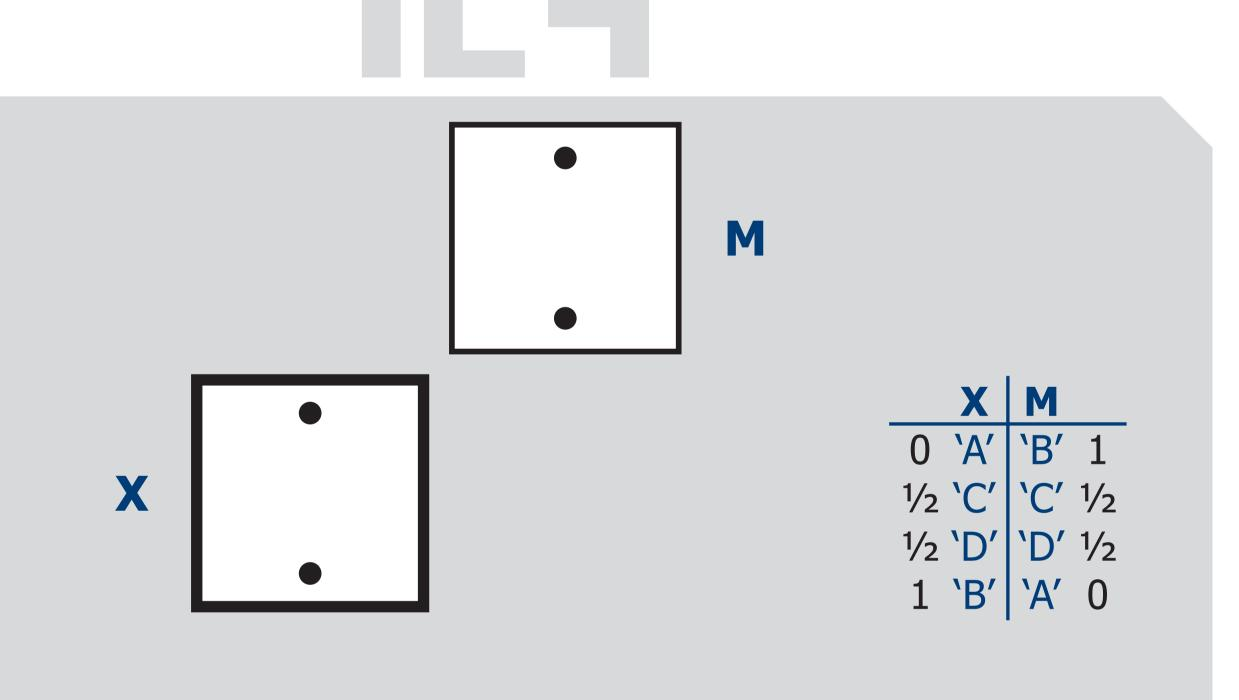
The inverter. The logic values 0 and 1 enforced to the driver appear inverted in the target cell, whereas the logic value  $\frac{1}{2}$  retains the same configuration.
