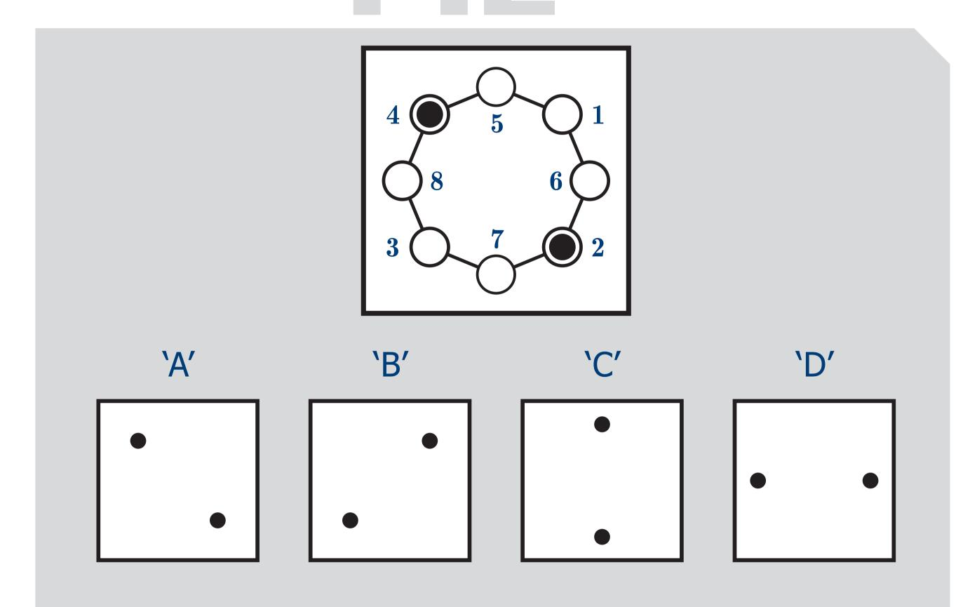
The extended quantum-dot cell with eight quantum dots separated with tunneling barriers. Owing to electrostatic repulsion the two electrons tend to align along one of four distinct configurations that correspond to their maximum spatial separation.
